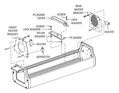
Figure 1. Heater and Defroster Kit Installation
